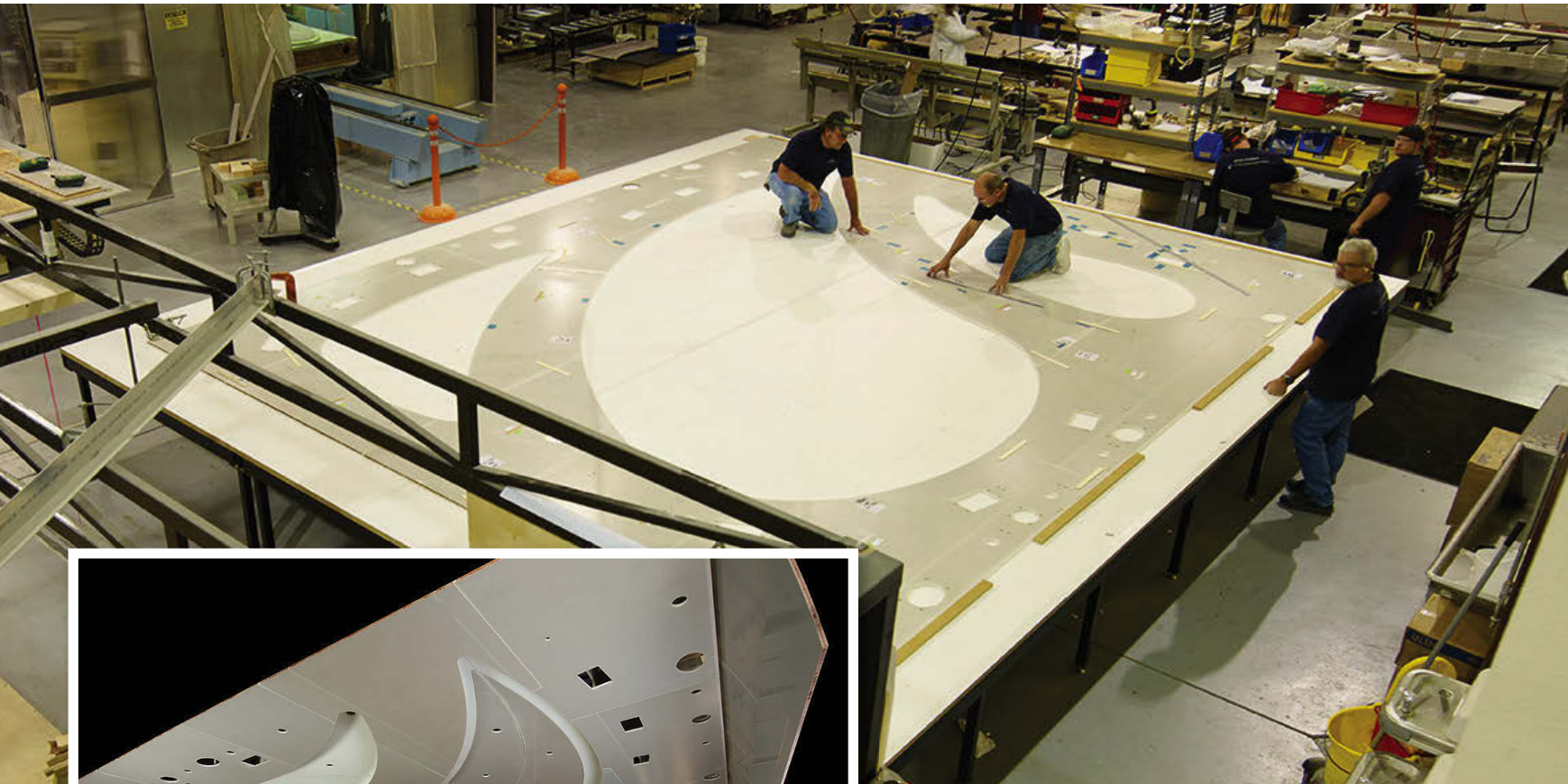
Initial layout of 747-8 Ceiling Panel Assembly at Jormac Aerospace
