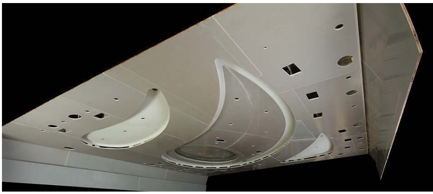
747-8 Ceiling panel assembly during fit check in full-scale mockup
