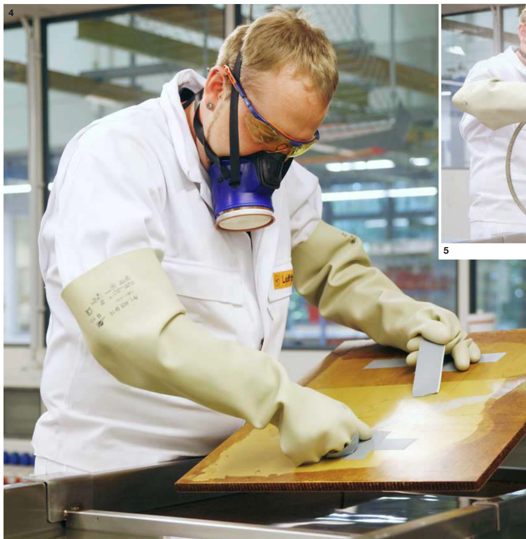
4-6. The wet film transfer process at Lufthansa Technik
