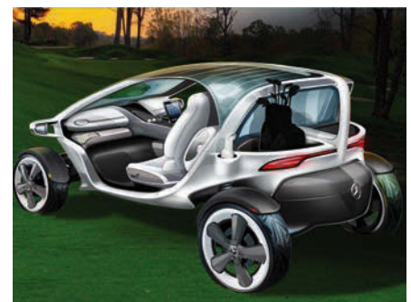
The Mercedes-Benz Vision Golf Cart concept, which includes Bluetooth connectivity, heated and ventilated seats, a neck-level heating system and lots of stowage
