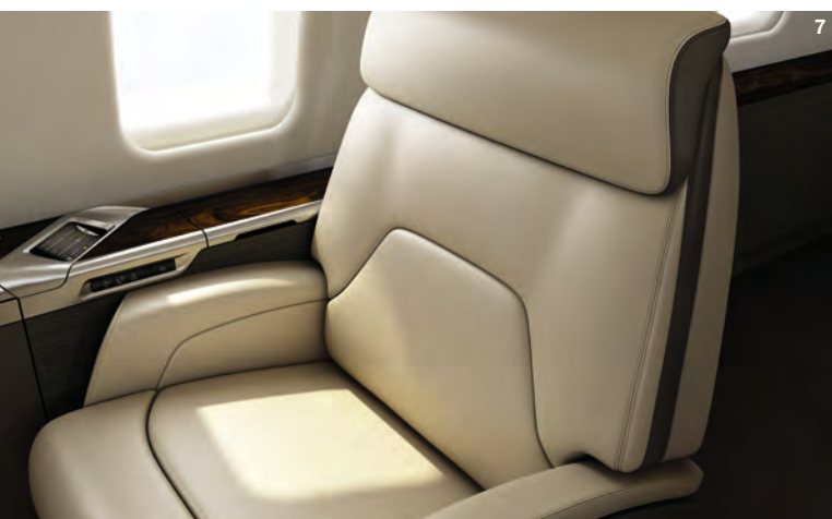
7. Bombardier's new seat for the Challenger 650 has a larger seat pan and an adjustable headrest
