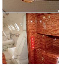
dispenser. The drawer cabinet has a 0.5ft<sup>3</sup> storage drawer and a 2ft<sup>3</sup> shelf area. The lavatory can be isolated for privacy with a solid partition that deploys between the cockpit and airstair door, and the cabin and the entryway. The Hiller cabinets can be painted or finished in the customer's choice of Carl Booth veneer.
