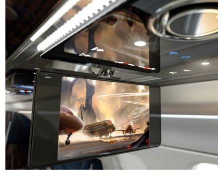
ABOVE: READING LIGHTS ON THE PHENOM 300E ARE INTEGRATED IN THE UPPER TECHNOLOGY PANEL. THE CONTROLS LIGHT UP WHEN A HAND IS DETECTED NEARBY
