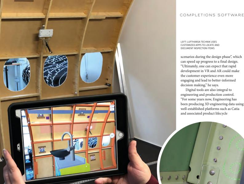
This approach minimizes risk by highlighting design issues before building the product. "Even in the empty aircraft, through the eye of the tablet and ahead of time, you can see the stowage, seat or any other interior part that will be installed."
