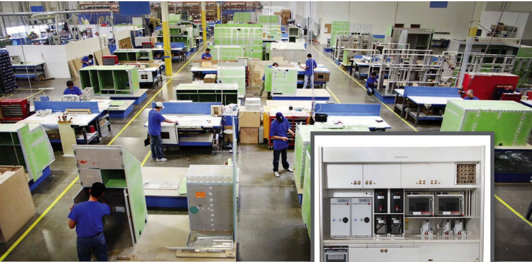
Airbus and Boeing VIP and VVIP Galleys under construction at Cabin Innovations
