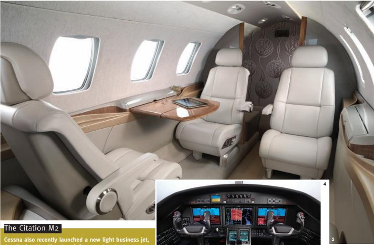
Cessna also recently launched a new light business jet, the Citation M2. The aircraft features Garmin G3000 avionics, engines similar to those on the Citation CJ series and an all-new interior design. A cabin mock-up was displayed alongside the Citation Latitude at NBAA 2011. The Citation M2's first flight is scheduled for the first half of 2012, with FAA certification (Part 23) expected in the first half of 2013, followed by deliveries beginning in the second half of 2013.
