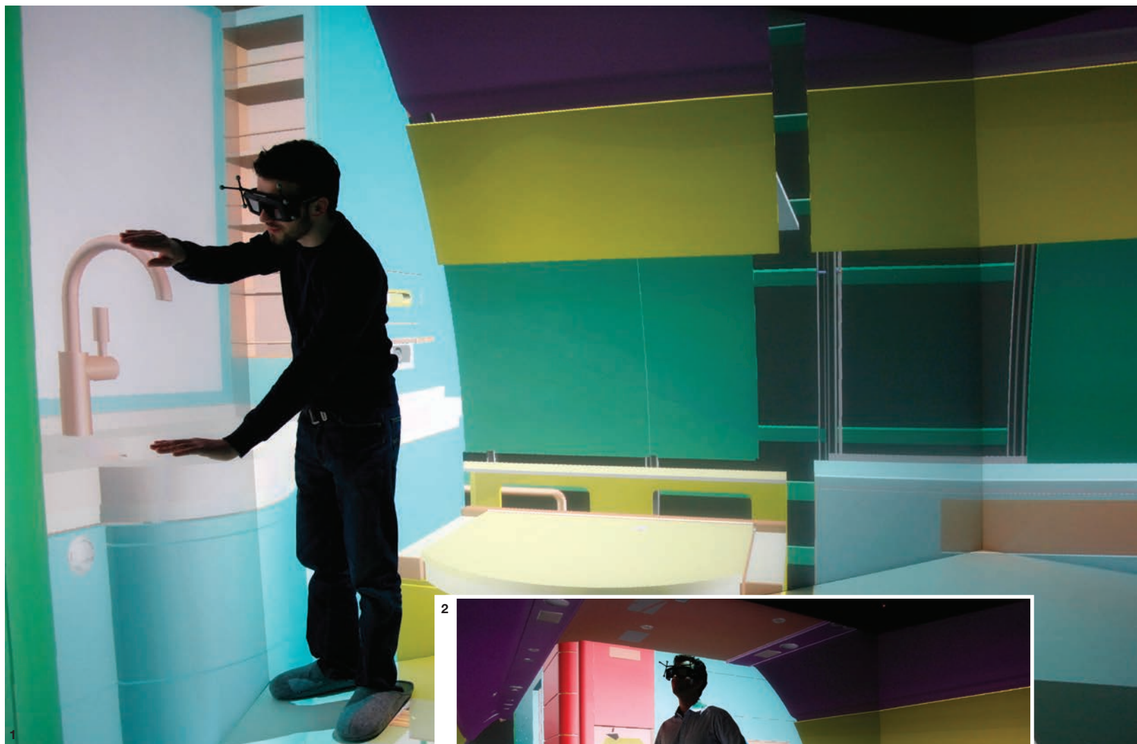
1-2.CAVE allows designers and technicians to step into the cabin virtually
